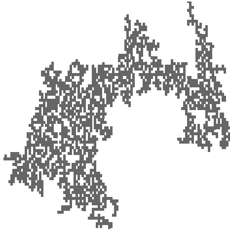
Fig. 6.35. Example of a cluster of invaders obtained on a square lattice after 2000 iterations of the invasion rule.
